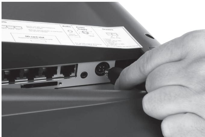
Fig. 24: Unplugging the power plug
