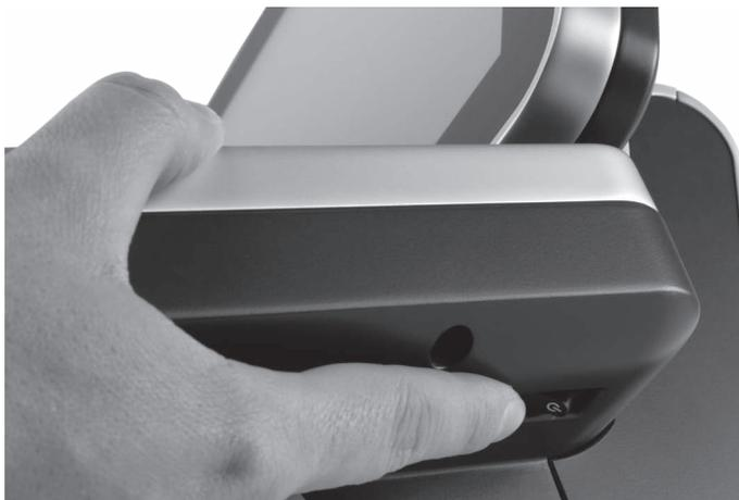
Fig. 22: Switching on and off Vario II
