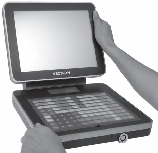
Fig. 15: Adjusting the display
