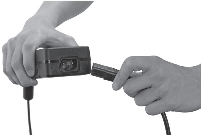
Fig. 25: Unplugging the female connector
