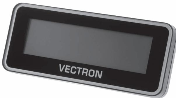
Fig. 27: Customer display Vectron C56
