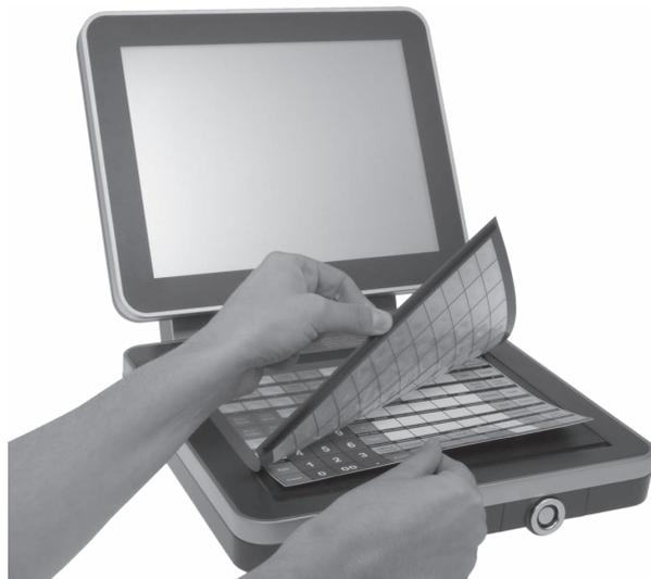
Fig. 14: Lifting the keyboard film and aligning the insert
