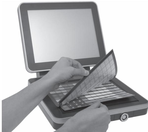
Fig. 26: Lifting the keyboard film and aligning the insert
