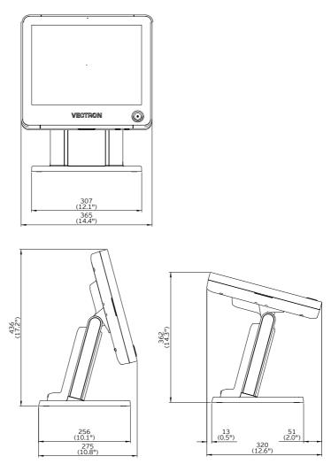
Fig. 4: POS Touch 15 Dimensions incl. foot S420 (in mm and inch)
