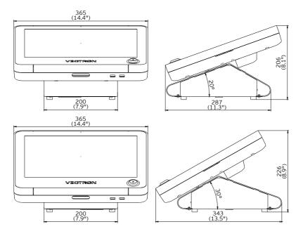
Fig. 5: POS Touch 15 Dimensions incl. foot S500 (in mm and inch)
