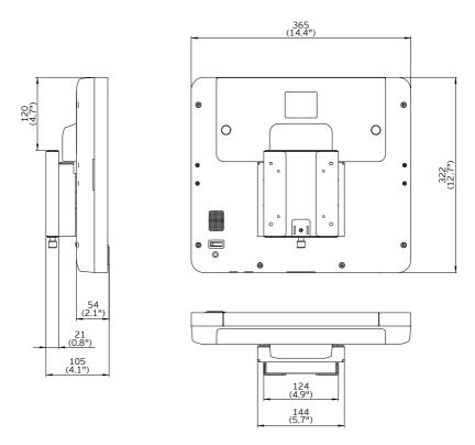
Fig. 6: POS Touch 15 incl. wall mount (in mm and inch)
