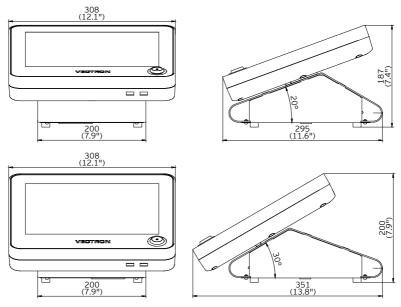
Fig. 5: POS Touch 12 Dimensions incl. foot S500 (in mm and inch)
