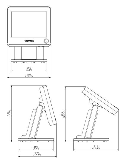
Fig. 4: POS Touch 12 Dimensions incl. foot S420 (in mm and inch)
