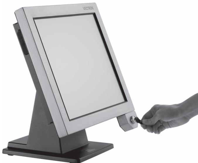
Fig. 15: Removing the key from the operator lock
