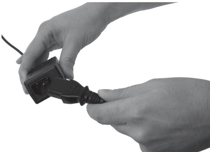
Fig. 55: Unplugging the female connector from the mains plug
