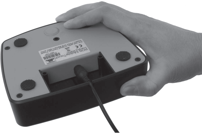
Fig. 13: Putting the plug to the female jack
