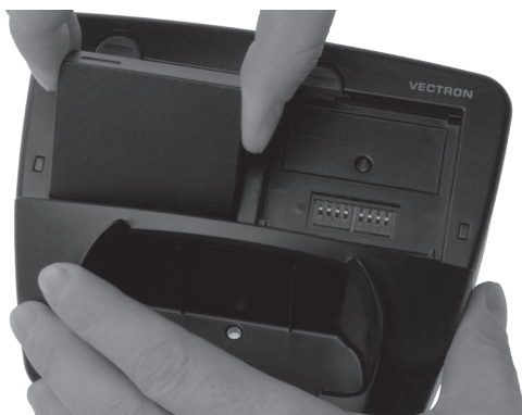
Fig. 15: Inserting the B50 to the battery compartment
