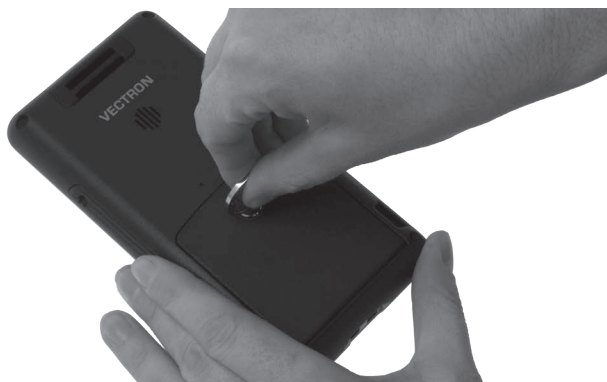
Fig. 17: Releasing the battery compartment screw
