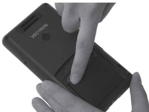
Fig. 20: Locking in the battery B50
