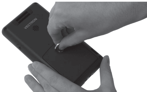
Fig. 46: Fastening the battery compartment screw
