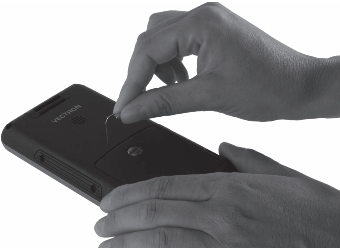
Fig. 48: Pressing the reset key
