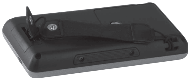
Fig. 25: Pushing the loop through the lug and the push button through the loop
