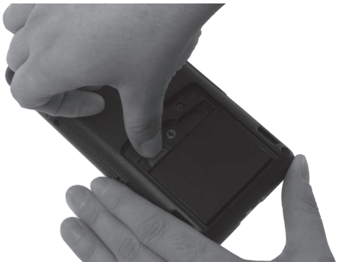
Fig. 43: Enabling the battery release
