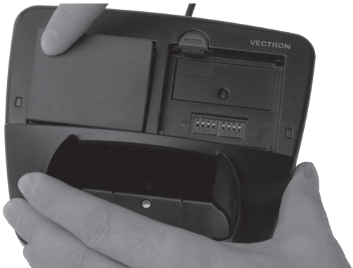
Fig. 16: Locking in the battery B50
