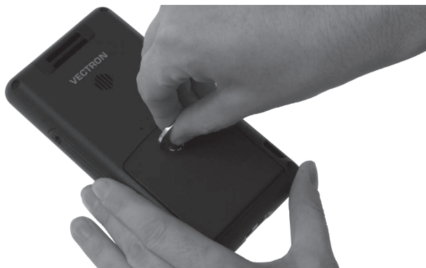
Fig. 50: Releasing the battery compartment screw
