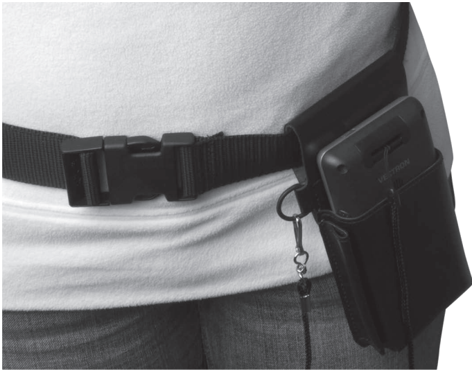
Fig. 37: Putting the MobileTouch into the leather holster
