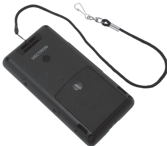
Fig. 29: Pushing the safety strap through the loop
