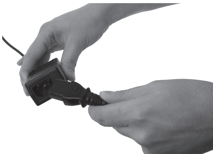
Fig. 14: Putting the female connector to the mains plug
