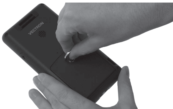
Fig. 21: Fastening the battery compartment screw
