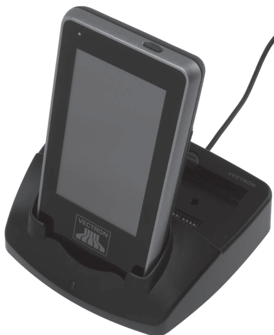
Fig. 22: Inserting the MobileTouch to the charging station
