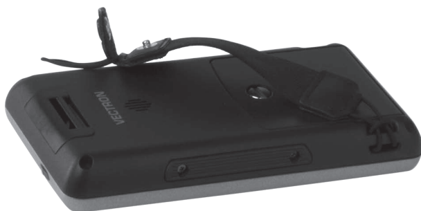
Fig. 24: Pushing the wrist strap through the loop
