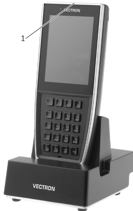
Abb. 22: POS MobilePro III in Ladestation
