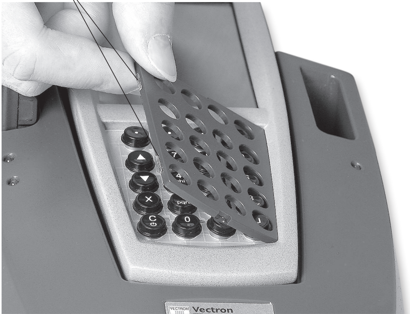
Fig. 29: Inserting the keyboard grid
