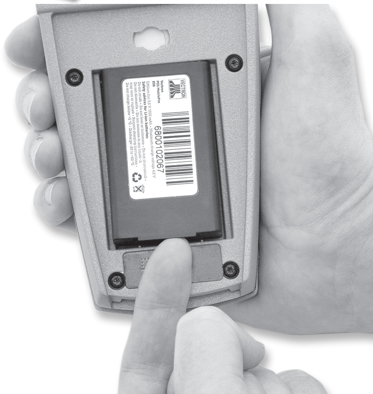
Fig. 8: Lifting the battery
