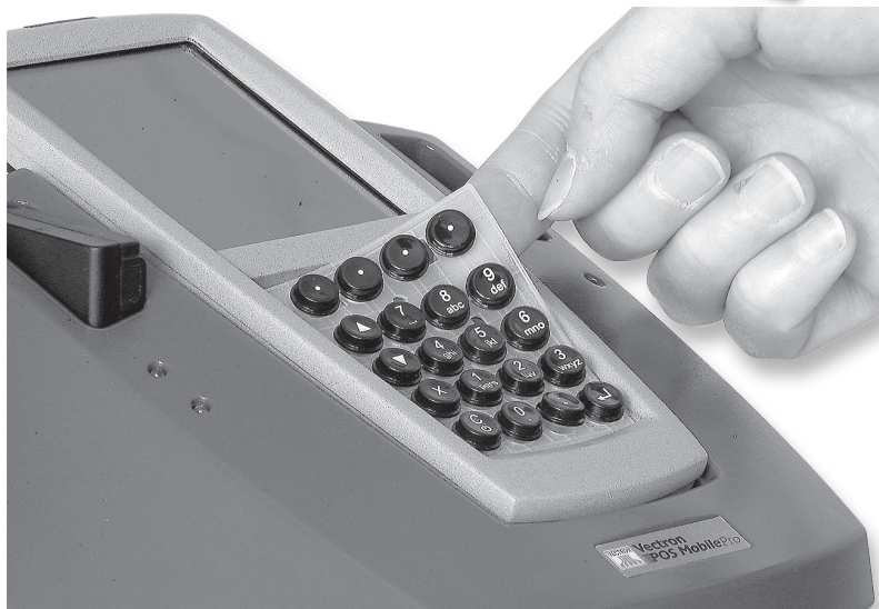
Fig. 26: Removing the keyboard pad
