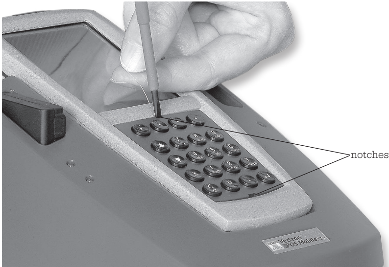
Fig. 23: Lifting the keyboard grid
