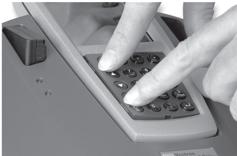
Fig. 30: Fixing the keyboard grid
