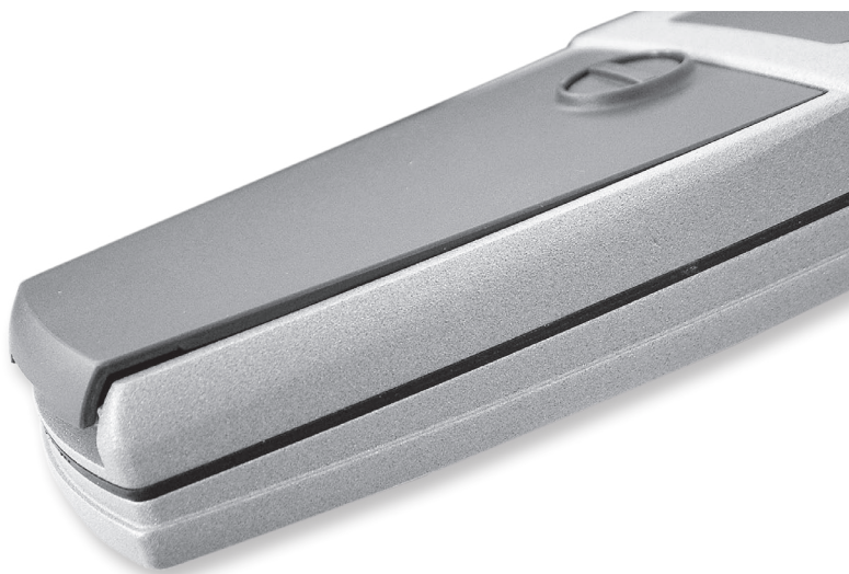
Fig. 13: Battery lid is not closed correctly
