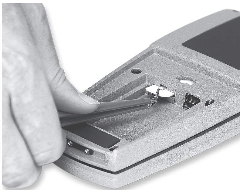
Fig. 17: Removing the SIM-card
