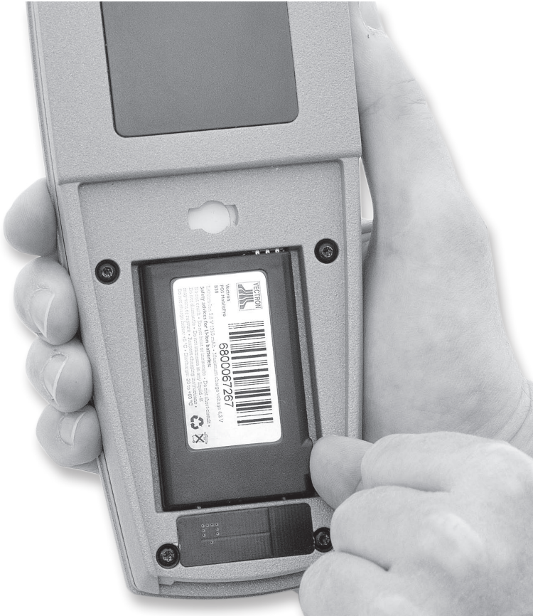
Fig. 7: Lifting the battery
