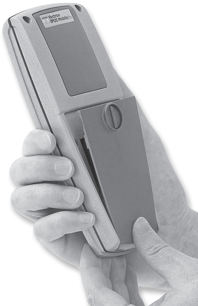
Fig. 5: Lifting the lid
