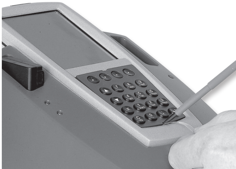
Fig. 24: Lifting the keyboard grid
