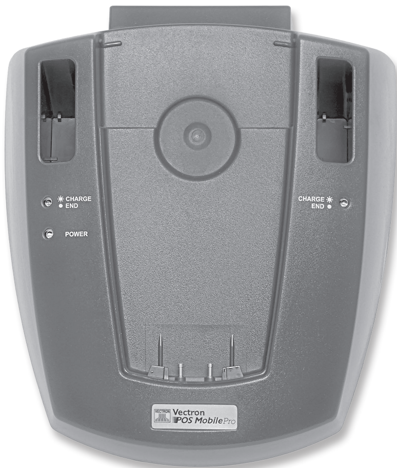
Fig. 19: Charging station for Vectron POS MobilePro
