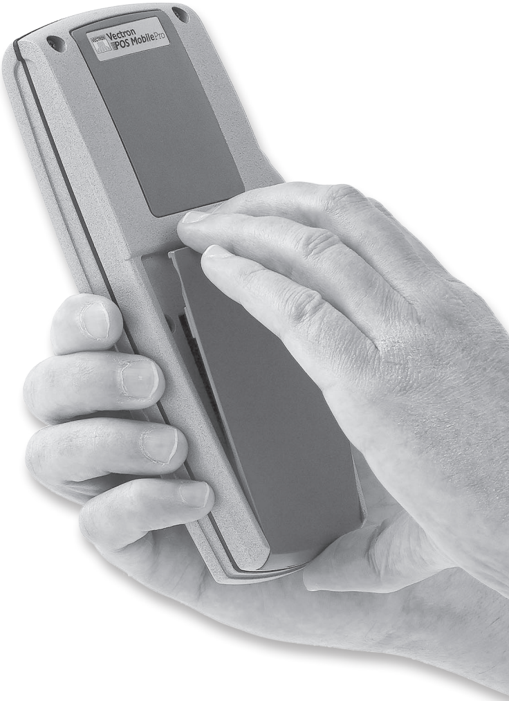
Fig. 6: Removing the lid
