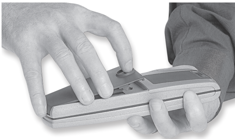
Fig. 12: Closing the battery compartment lid
