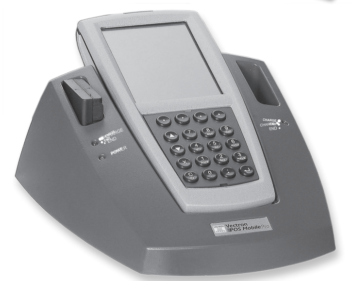
Fig. 20: Terminal and one battery in charging station
