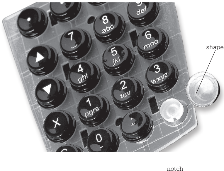
Fig. 28: Putting on the key caps
