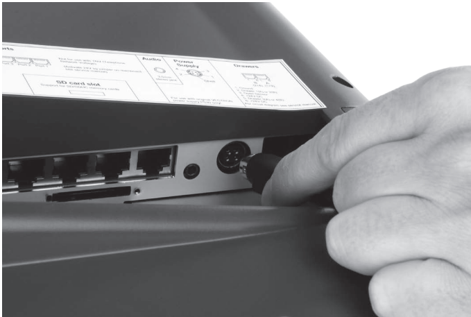
Fig. 12: Putting the power cable plug to the power connection
