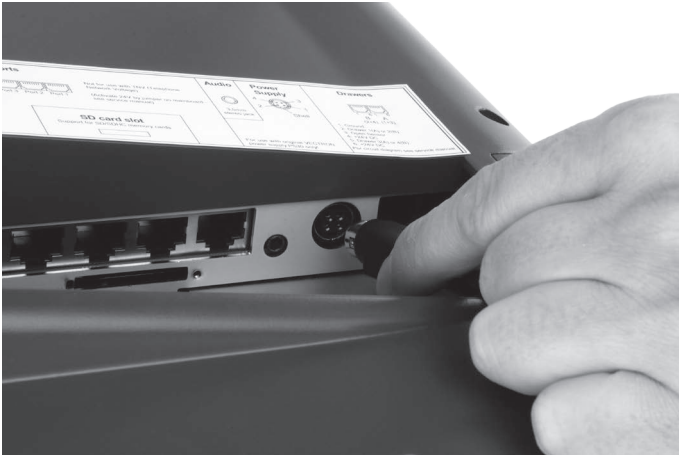
Fig. 24: Unplugging the power plug
