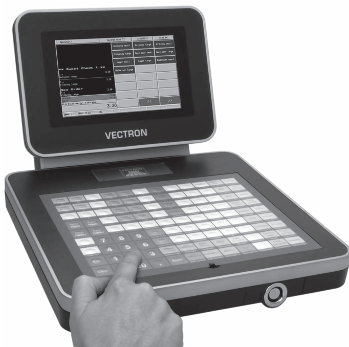
Fig. 18: Entering data via flat keyboard
