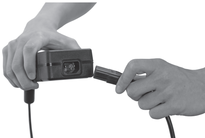
Fig. 25: Unplugging the female connector
