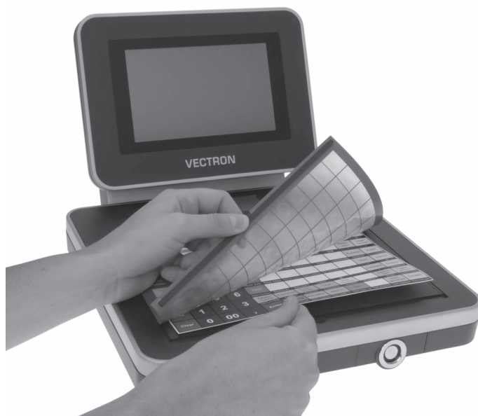
Fig. 14: Lifting the keyboard film and aligning the insert
