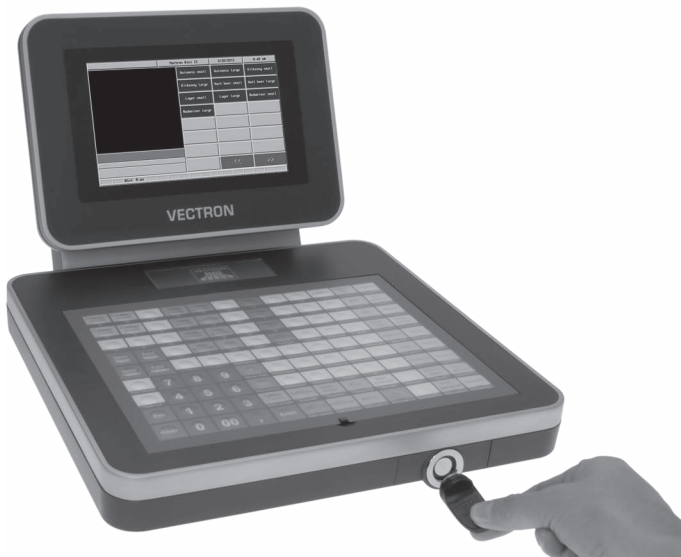
Fig. 21: Approaching and removing the key
