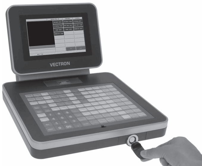
Fig. 20: Approaching the key to the operator lock
