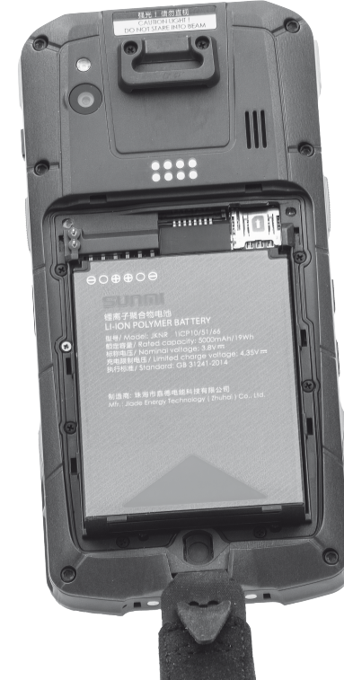
Fig. 16: Inserting the battery
