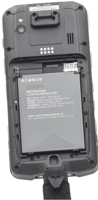
Fig. 18: Battery compartment lid removed
