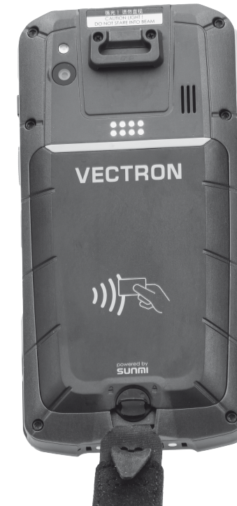
Fig. 12: Opening the locking of the battery compartment lid
