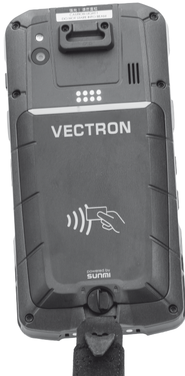
Fig. 13: Opening the locking of the battery compartment lid
