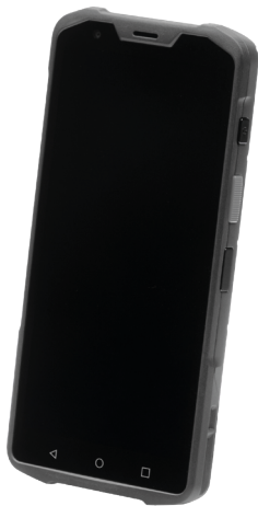
Fig. 6: Vectron POS M4 PAY 74.6 x 154.4 x 17.1 mm (2.9 x 60.8 x 6.7 inch)
