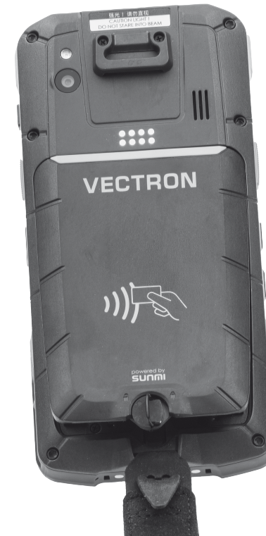
Fig. 14: Opening the battery compartment lid
