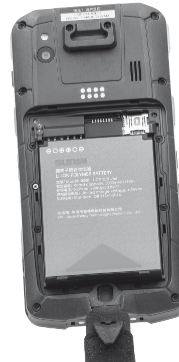
Fig. 19: Pulling the battery to the top
