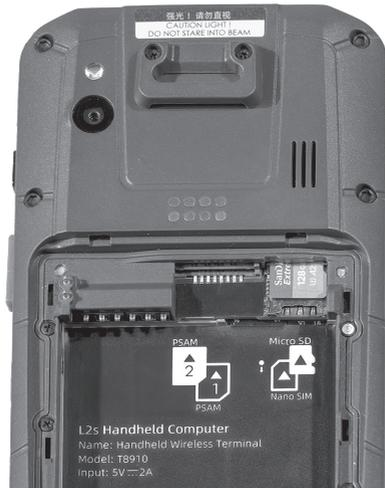
Fig. 23: MicroSD card inserted
