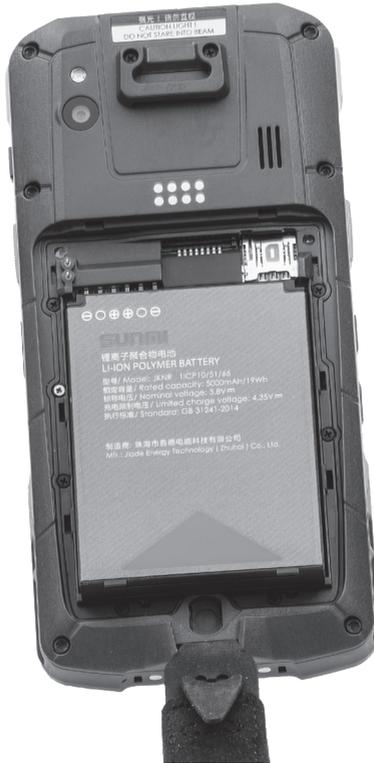
Fig. 16: Inserting the battery
