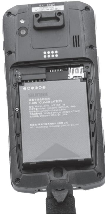
Fig. 19: Pulling the battery to the top
