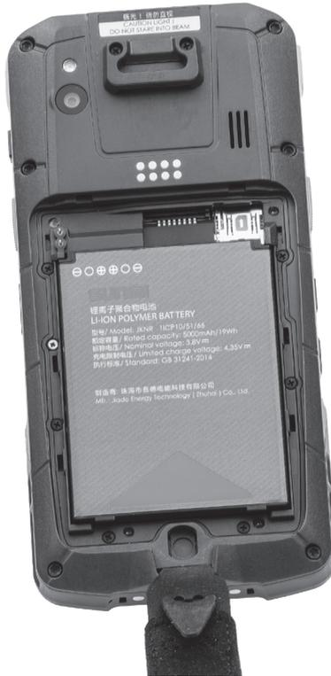
Fig. 17: Inserted battery
