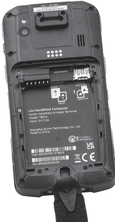
Fig. 15: Battery compartment lid removed
