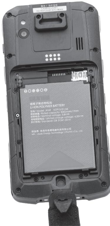
Fig. 18: Battery compartment lid removed
